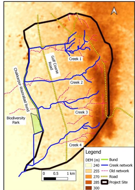
The Golf Course Road is at an average elevation of 250m, while the bund at 245m and Paras hospital and Sheeba apartment are at 240m. Hence, being low-lying spots, these form the chronic flooding spots.
